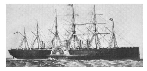
L \* B \* D = 211m \* 36m (over the paddle boxes) \* 9.2m with 18m height of hull. Propulsion: Four steam engines for the paddles and an additional engine for propeller. Total power estimated 6.0 MW
