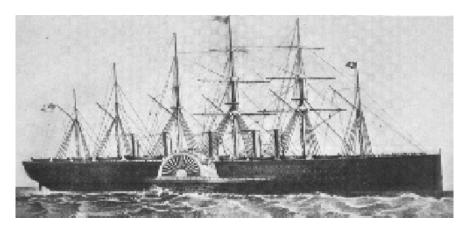
L \* B \* D = 211m \* 36m (over the paddle boxes) \* 9.2m with 18m height of hull. Propulsion: Four steam engines for the paddles and an additional engine for propeller. Total power estimated 6.0 MW
